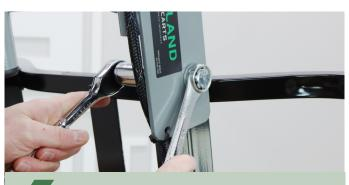
Install a washer and nut onto the bolt and tighten down using a 3/4" wrench and socket.
