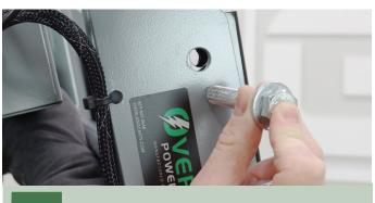
Align the handle over the holes and insert the bolts and washers to hold it in place.
